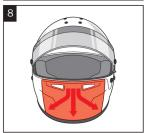
8. Using a soft cloth or microfiber cloth, to press the new chin guard against the helmet chin bar from top to bottom and sides to secure proper bonding between the two parts.
