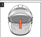
3. Without removing the adhesive strips on the back of the chin guard, place the chin guard on the helmet chin bar to self-center the part in the middle.
