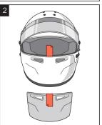
2. Prepare two pieces of masking tape and select a pen or marker. Open the shield and apply one piece of tape in the middle of the upper chin bar and another in the middle of the upper chin guard.
