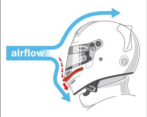
Center the Chin Bar Gurney just below the chin bar vents and mark points of reference. Remove the protection tape from the adhesive and place the Chin Bar Gurney on the helmet starting from the middle and let it fall in position (avoid tension). Press firmly on the edges for good adherence.
