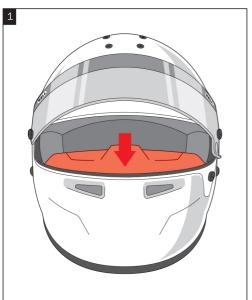
**1.** Insert the breath deflector between the shell and the face piece, with the protruding center facing outwards.
