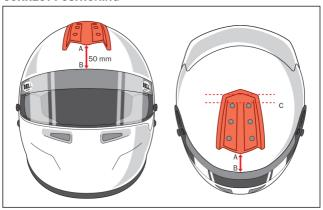
Place the Air intake at approximately 50 mm from the visor (A to B), and center it over the aeration holes (C). To avoid lift, do not place the Air Intake higher than indicated above.
