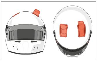
Before installing the Forced Air insert and the Cover Plate, remove the protective cover from the back side of the Forced Air insert and the Cover Plate exposing the adhesive material that will seal the Forced Air insert and the Cover Plate to the helmet shell. Once installed press firmly around the edges of the Forced Air insert and the Cover Plate to assure proper adhesion.
