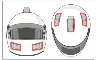
Place the Forced Air and Cover Plate Seals on top of the Forced Air inserts or on top of the Cover Plates to ensure a perfect seal and prevent air escaping or entering.
