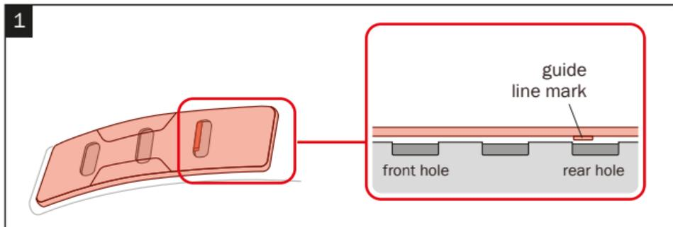
Place the Forced Air and Cover Plate Seal on top of the Cover Plate to ensure a perfect seal and prevent air from entering.
