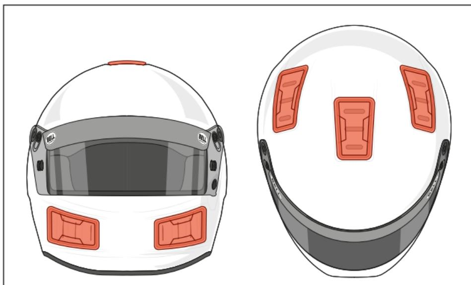
Before installing the Cover Plate, remove the protective cover from the back side of the Cover Plate exposing the adhesive material that will seal the Cover Plate to the helmet shell. Once installed press firmly around the edges of the Cover Plate to assure proper adhesion.
